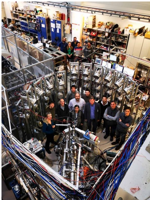
Left: MONSTER neutron spectrometer developed by CIEMAT. Right: n_TOF total absorption gamma-ray calorimeter used at CERN for neutron capture cross section measurements.
